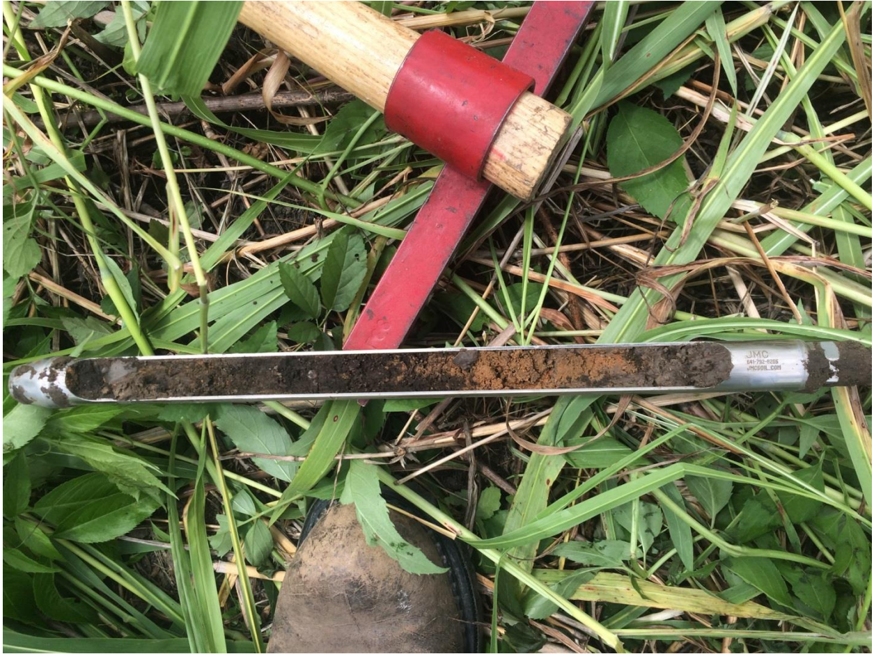
Figure 22 Typical burned surface as expose in the core tube.
