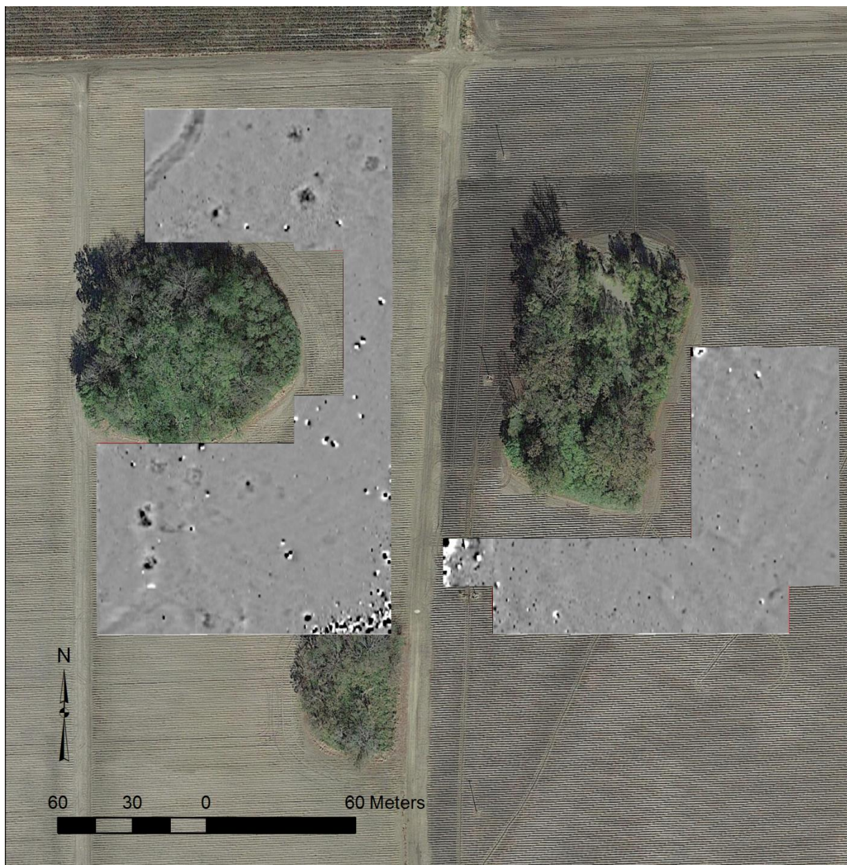
Figure 3 Arcola, gradiometer image and recent aerial image.
